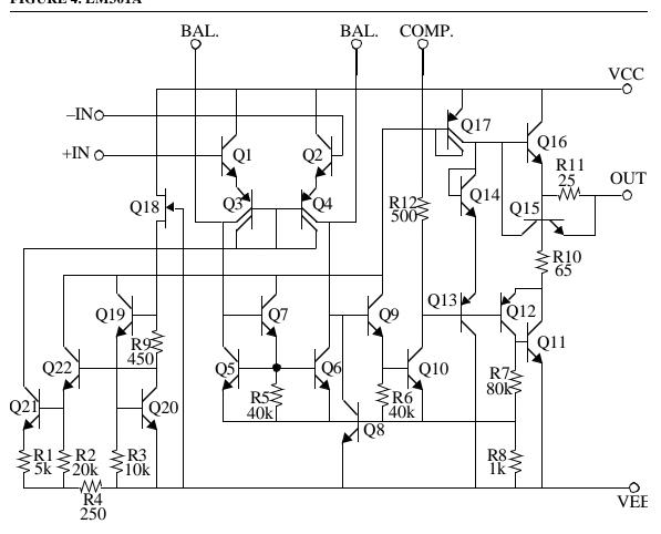
Another change, enabled by process improvements that produce higher PNP  $\beta$ , is simplified biasing of Q3/Q4 and Q17. The multiple collectors may be thought of as a shorthand notation for mirrors, where the current ratios are set by collector area ratios. Finally Q18,
