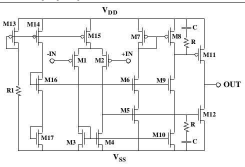
Here, M13-M15 establish the bias currents for the amplifier, while the stack of M16 and M17 provide a bias voltage for common-gate cascode devices M6 and M9.
