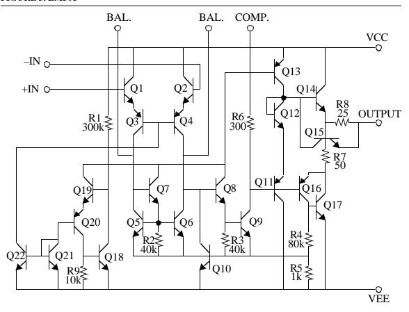
To improve input common-mode range, Widlar had to develop a more satisfactory solution to the level shift problem. A battery-based shifter, after all, more than simply re-centers the common-mode level; it also necessarily subtracts from it. The traditional alternative to a battery is simply to alternate NPN- and PNP-based stages, where the downward common mode shift of the latter compensates for the upward shift of the former.
