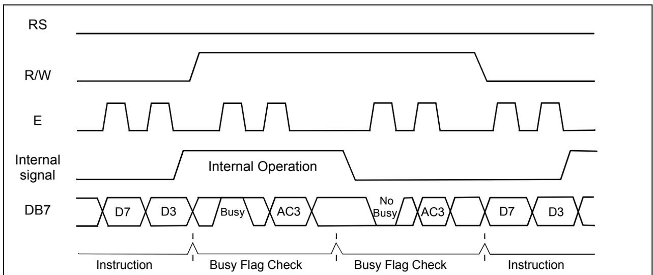
**Figure 5 . Example of 4-bit Bus Mode Timing Diagram**
