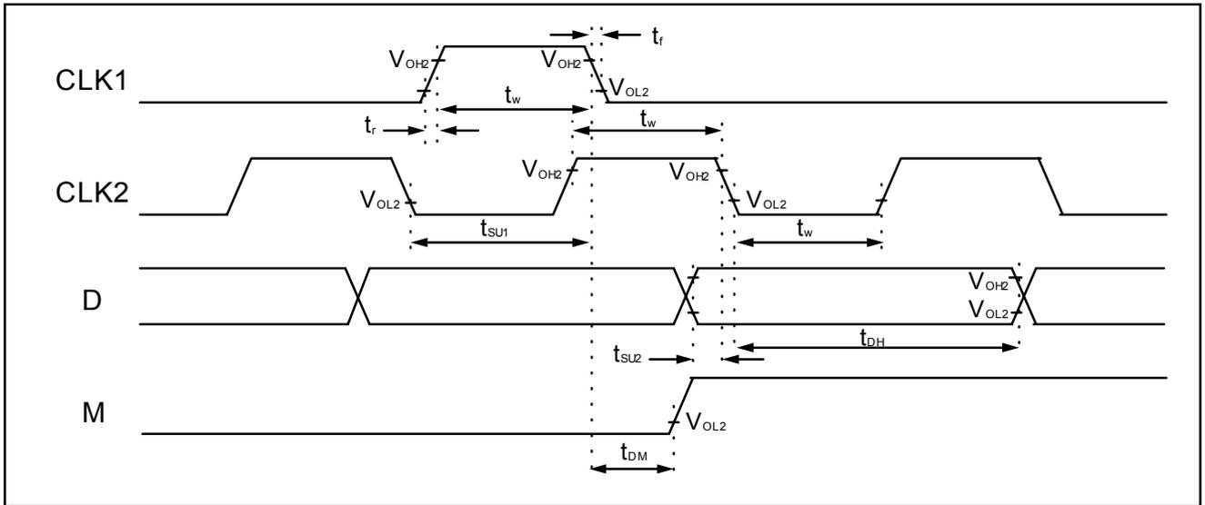
Figure 8 . Interface Mode With Extension Driver Timing Diagram
