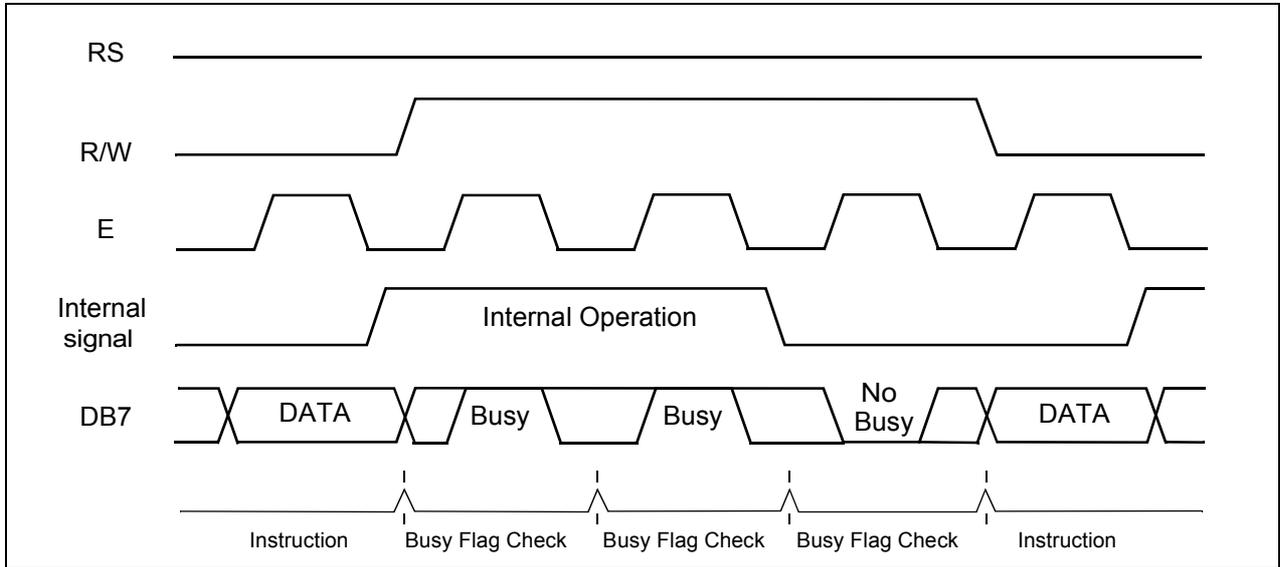
**Figure 4 . Example of 8-bit Bus Mode Timing Diagram**
