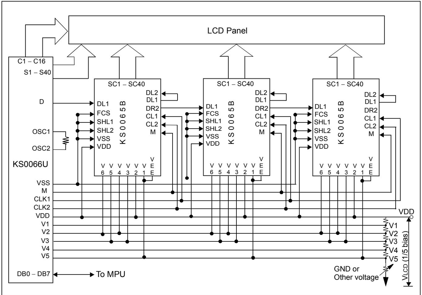
NOTE: When KS0065B is externally connected to the KS0066U, you can increase the number of display digits up to 80 characters.
