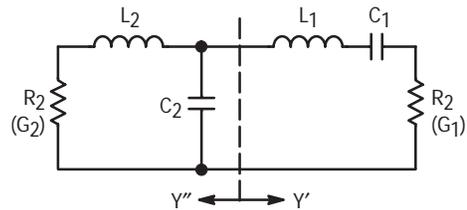
$$Y' = G' + jB' = \frac{R_1}{R_1^2 + (\omega L_1 - 1/\omega C_1)^2} - \frac{j(\omega L_1 - 1/\omega C_1)}{R_1^2 + (\omega L_1 - 1/\omega C_1)^2}$$
