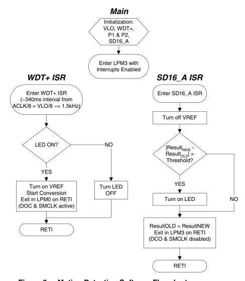
Figure 3. Motion Detection Software Flowchart
