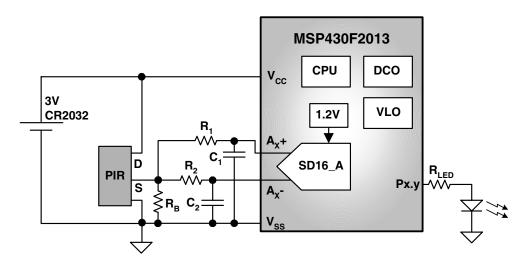
Figure 1. MSP430F2013 Motion Detection System
