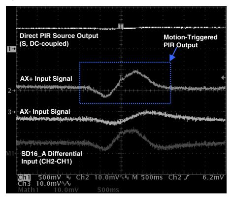
Figure 2. PIR Sensor Output & Signal Conditioning
