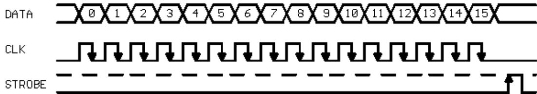
Data input to the serial pin are 16-bit data transferred from DATA 0 to DATA 15.
