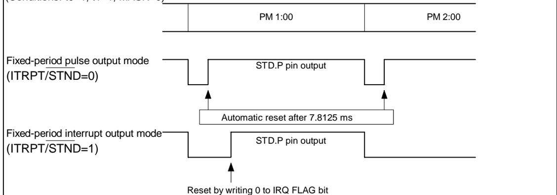
**iii. Frequency of STD.P pin output in fixed-period pulse output mode**
