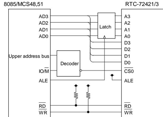
The resistors on the RD and WR lines are not necessary if the CPU does not have a HALT or HOLD state.
