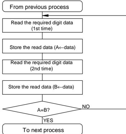
The operation when the HOLD bit is not used involves reading the same digit twice and comparing the read values. This is to avoid the problem of reading unstable data that would occur if the data was read while the RTC was incrementing the count.
