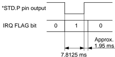
The output levels of the STD.P pin are low (down) and open circuit (up).
