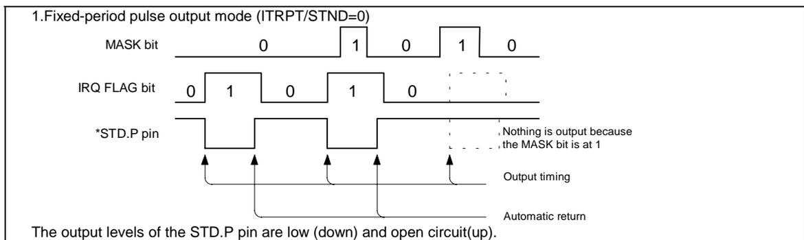
The output levels of the STD.P pin are low (down) and open circuit (up).
