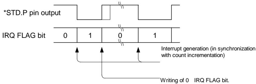
The output levels of the STD.P pin are low (down) and open circuit (up).
