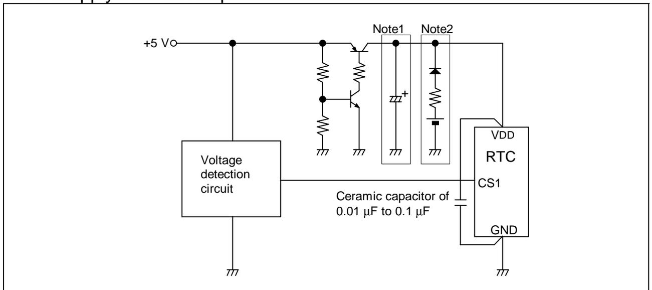
Note 1: This capacitor must be of a high capacity because a transient reverse current flows from the collector to the emitter of the transistor when the power is turned off.
