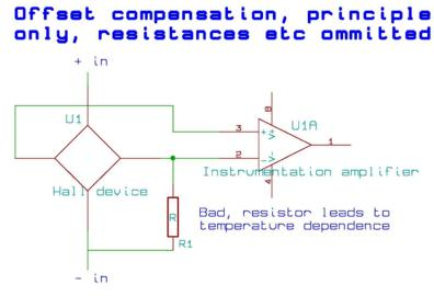
The example above leads to a temperature drift of the offset voltage. Meaning that the offset voltage is not constant but changes with temperature and is difficult to compensate.
