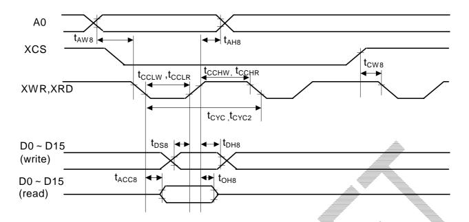
Be sure not to alternate the signal XCS and/or A0 when XWR="L" or when XRD="L".
