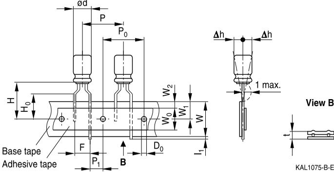
**Lead spacing 5.0 mm ( $\varnothing d = 10 \dots 12.5$  mm)**
