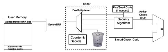
Figure 9: Adding Fourth Output to De-Multiplexer
