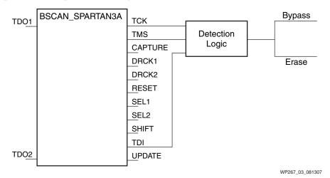
Figure 4: Detection Logic
