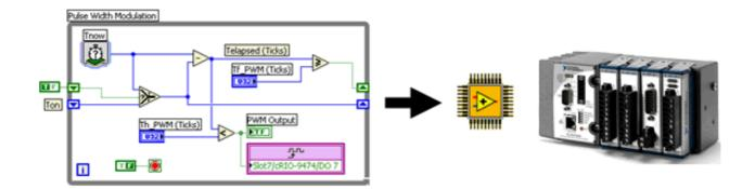
With the embedded RIO FPGA hardware, you can implement multiloop analog PID control systems at loop rates exceeding 100 kS/s. Digital control systems can be implemented at loop rates up to 1 MS/s, and it is possible to evaluate multiple rungs of Boolean logic using single-cycle while loops at 40 MHz (25 ns). Due to the parallel nature of the RIO core, adding additional computation does not necessarily reduce the speed of the FPGA application.
