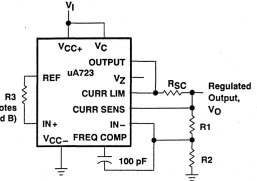
**Figure 2. Basic High-Voltage Regulator**
