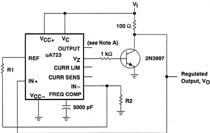
NOTE A: When 10-lead uA723U devices are used in applications requiring  $V_Z$ , an external 6.2-V regulator diode must be connected in series with OUTPUT.
