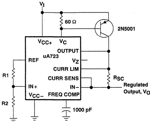
Figure 5. Positive-Voltage Regulator
