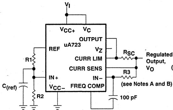
**Figure 1. Basic Low-Voltage Regulator**
