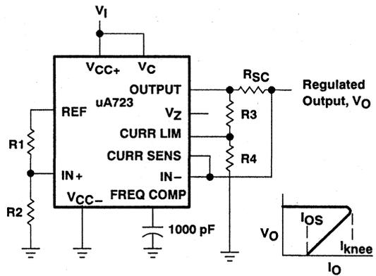
Figure 6. Foldback Current Limiting
