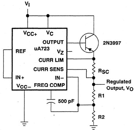
**Figure 4. Positive-Voltage Regulator**
