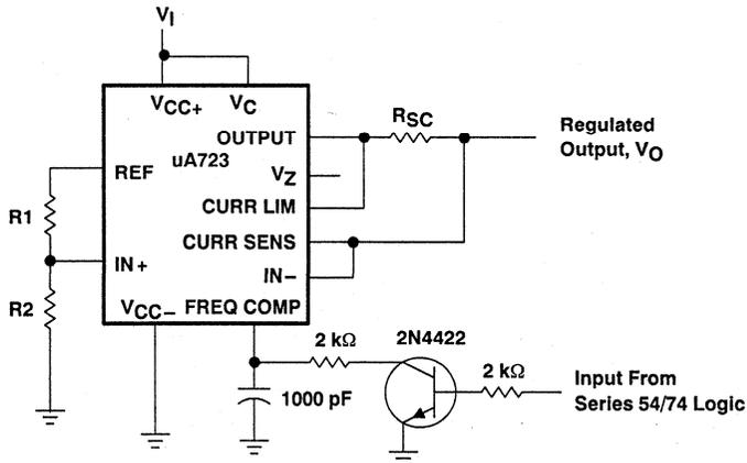
NOTE A: A current-limit transistor may be used for shutdown if current limiting is not required.
