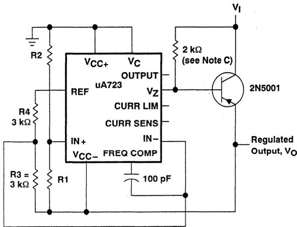
**Figure 3. Negative-Voltage Regulator**
