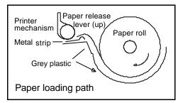
mechanism grips the paper and feeds it through. There is an optical sensor which "sees" the paper and will drive the motor for a predetermined time. If the paper fails to grip and advance the paper, withdraw the paper and try again. When it reappears above the rubber, press the paper feed button, and allow enough to feed through for good alignment, thread the paper through the exit slot and close the lid.
