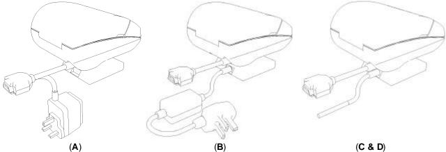
All four options are housed in the same type of replaceable pack, which clips into the underside of the printer and can be changed in a few seconds by the user. In each case, the primary power for the printer comes from this replaceable pack.
