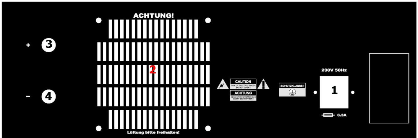
1. Connector for the power supply cable.
