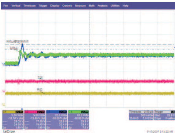
Figure 4. CANL Measured at Bus (Green) and Transceiver (Blue) at Short-Circuit Impact
