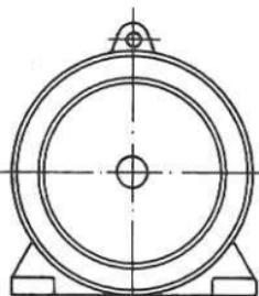
$$\begin{aligned}P &= 22 \text{ kW} \\n &= 1440 \text{ min}^{-1} \\M &= 150 \text{ Nm}\end{aligned}$$
