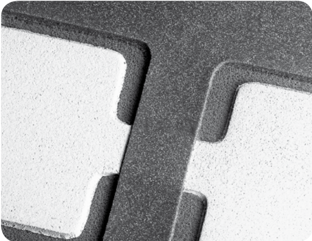
Low requirement of UV-exposure and fast developing, makes a solder-dam of 25 µ possible.
