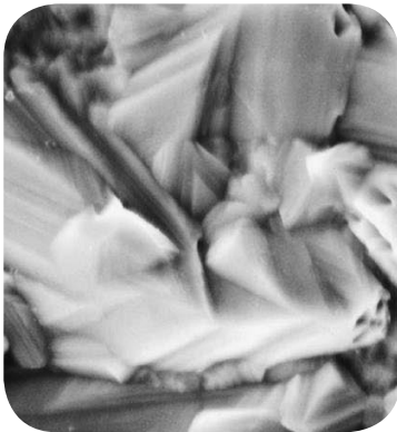
Large grain sized and dense packed crystals giving a pure white tin deposition for multiple solderability.
