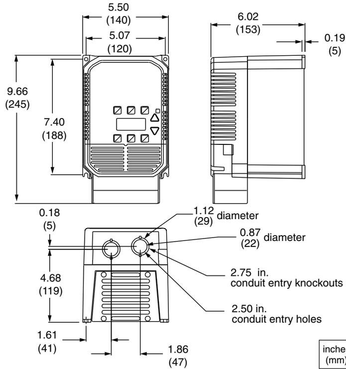
NOTE: On chassis models supplied without covers and conduit plates, depth = 5.81 (229).
