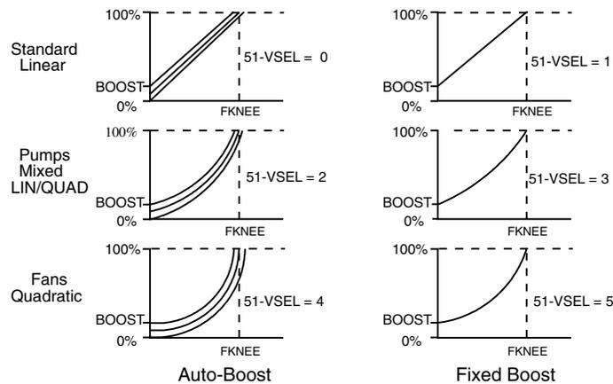
**Figure 14: V/Hz Characteristics**
