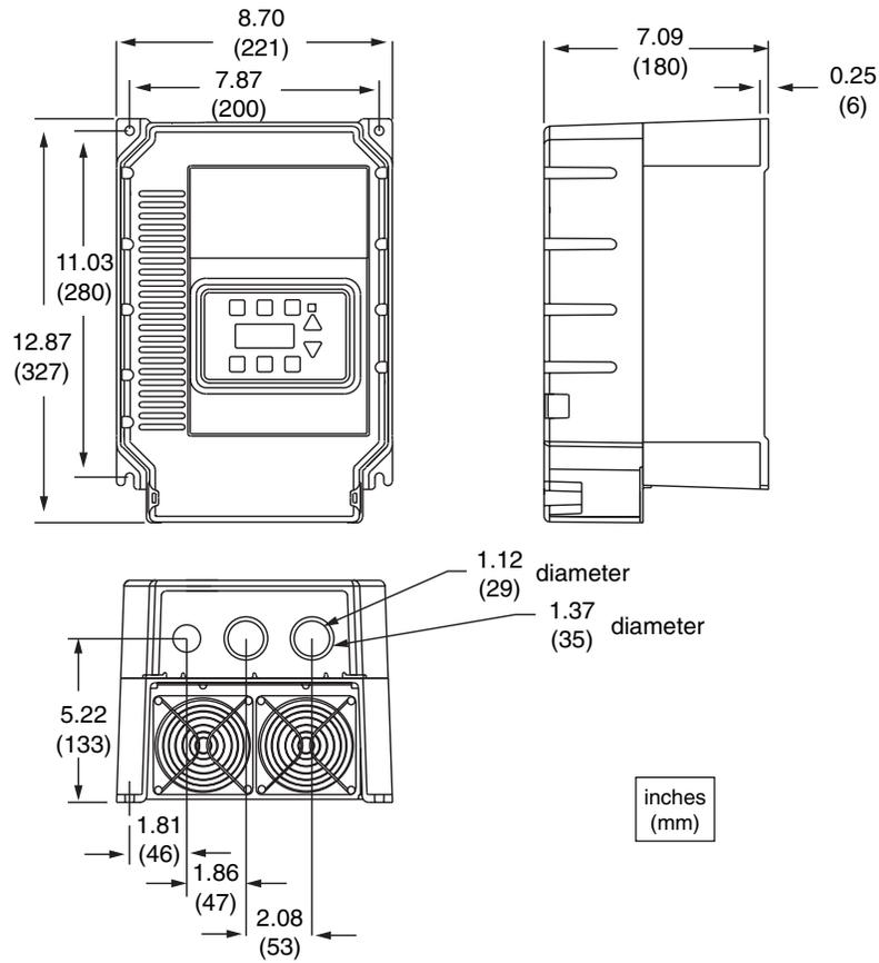
Figure 5: 7.5 to 20 HP 230 and 460 VAC, NEMA 1
