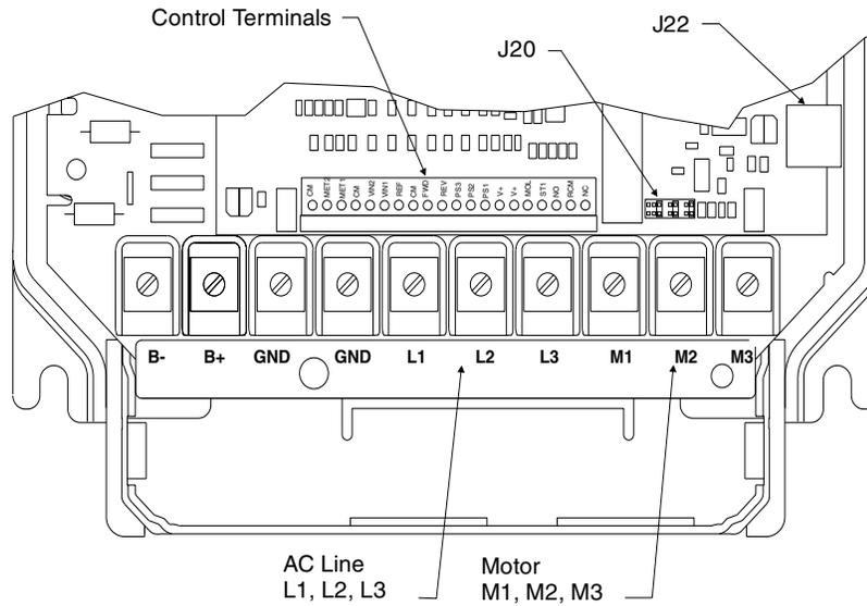
**Figure 10: Terminal Locations, 7.5 to 20 HP Inverters**
