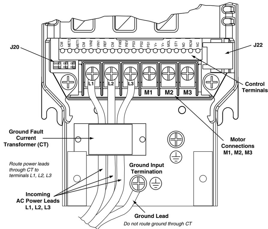
Figure 9: Terminal Locations, 0.5 to 5 HP Inverters
