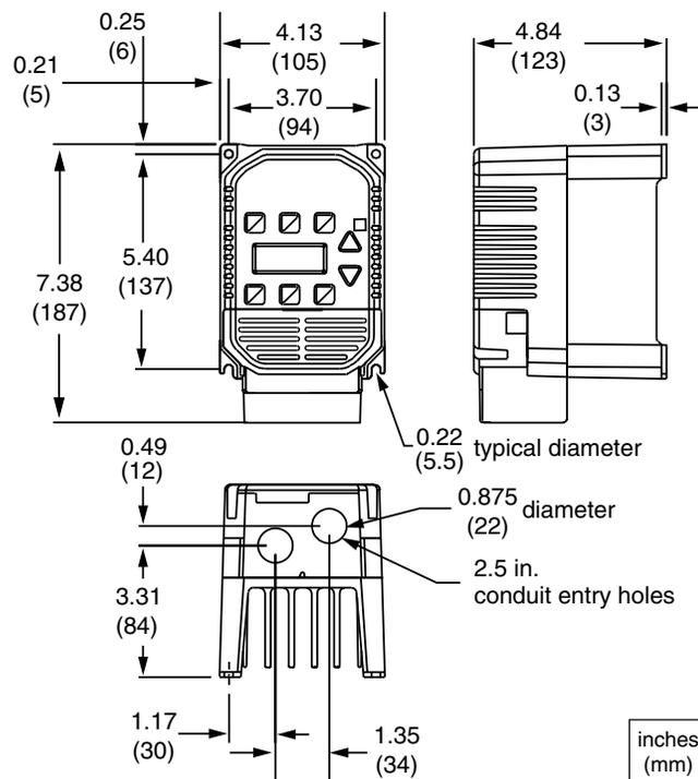
NOTE: On chassis models supplied without covers and conduit plates, depth = 4.68 (119).
