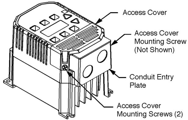
**Figure 7: Removing Cover From 0.5 to 5 HP NEMA 1 Inverters**
