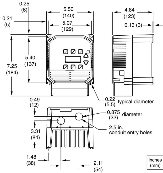
NOTE: On chassis models supplied without covers and conduit plates, depth = 4.68 (119).
