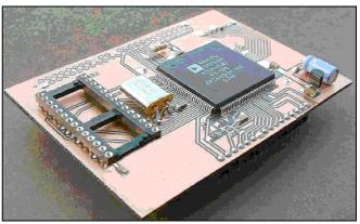
The finished Processor daughter board. Note that the crystal X3 is fitted after bending its leads - to reduce height. C120 and C121 are fitted under the board. IC26, when fitted in its socket defines the overall height of the complete DSP board.
