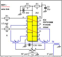
Fig 37: Two-transformer H-mode mixer by 17SWX. Details of transformer T6 (which replaces T4 and T5) will be provided next month. It is wound on the same ferrite as the other transformers.
