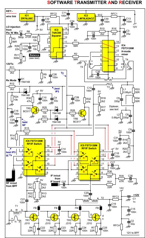
Fig 34: Dynamically configurable H-mode mixer - and quad J310 amplifier, better known as the 'Magic Roundabout'. The 'Rx Mode' line is set to +5V ie logic '1' for best intercept (IP3) - or to logic '0' for best noise figure (NF). 12VTx - when taken to +12V - selects the transmit configuration. The mixer requires fundamental frequency injection between -10 and +10dBm.
