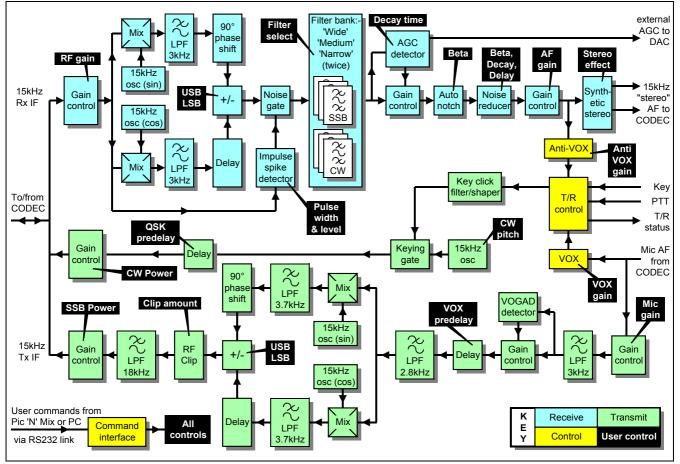
Fig 2: Software block diagram of PIC-A-STAR DSP functionality. Not shown are simple on/off switches associated with VOX, noise blanker, autonotch, noise reducer and the RF clipper. The filter bank also has an off (ie bypass) switch to give a net maximum bandwidth of some 3kHz.
