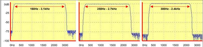
Fig 32: Plot of wide, medium and narrow Rx SSB filters. Other filters in the DSP receiver give a further theoretical 30dB of ultimate stop band. The pass-band ripple in all cases is less than 0.2dB. Because STAR is not a mere audio add-on, these widths are actually achievable - and useable.
