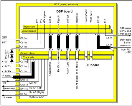
Fig 14: DSP sub-assembly. The IF board is bolted back-to-back to the DSP board using nuts, bolts and spacers. Both their groundplanes form a screen to isolate the two halves of the box. Feedthrough capacitors are used to route between the two halves of the box - and to the rest of the transceiver. C11 and C12 may be replaced with a stereo jack socket.
