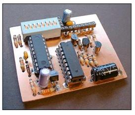
The Timer board, which will fit in a small corner in most transceivers and get rid of those DC switching relays.
