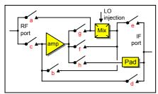
Fig 35: Magic Roundabout block diagram. For 'best NF', switches c, g and e are closed. For 'best IP3', switches a, b and h are closed and the pad improves the intercept. For 'transmit', switches d, f and a are closed.
