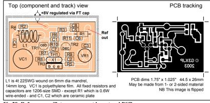
Fig 29: Reference oscillator component layout and PCB.
