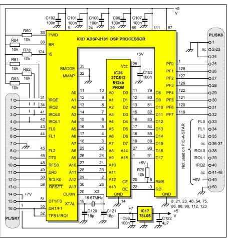
Fig 7: Processor daughter board circuit diagram. IC27 may be a KS-130 or KS-160 processor but in any event, the slower KS-130 device is assumed. To retain compatibility with EZLITE, the unused or unconnected lines on PL/SK8 are available on the mother board for non-STAR applications.
