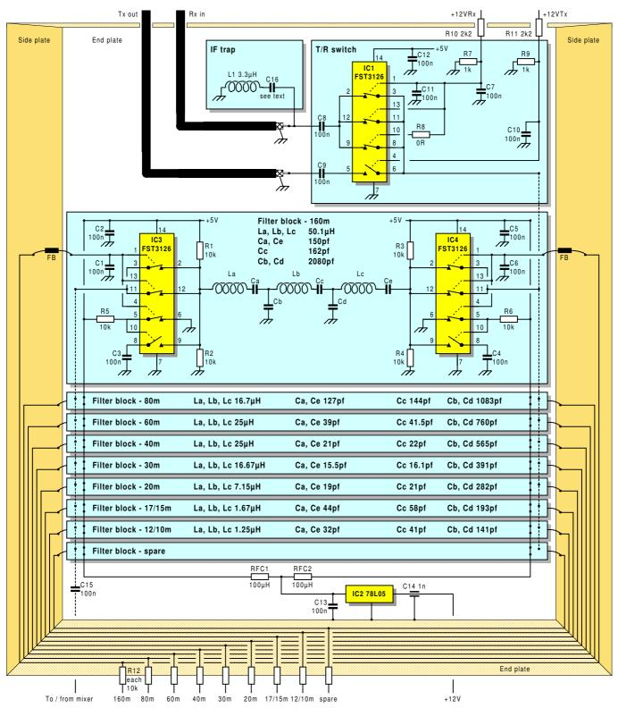
Fig 42: Band-pass filters circuit diagram and mechanical overview. All the filters have identical circuit diagrams. A band-select line is set to +5V to engage a filter block and to 0v to isolate it. This is compatible with direct interfacing to the Pic 'N' Mix band-select outputs. These lines are deliberately routed around the side-plates and *not* across the filter. For illustration, the 160m filter is shown 'on' and the T/R switch is 'on receive'.
