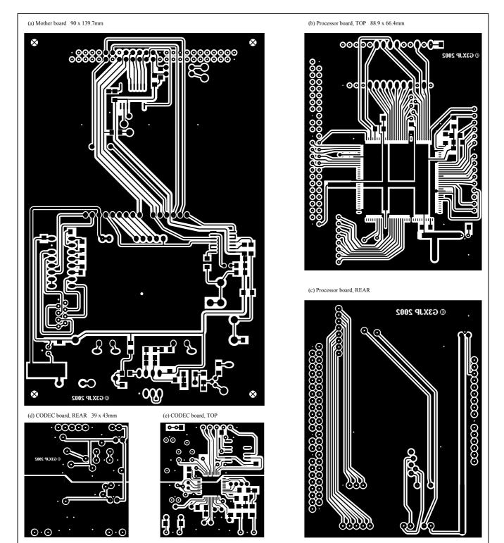
Fig 10: DSP boards PCB artwork. NB all these images are mirrored for direct copying to laser film. Should you wish to use an indelible pen to apply the artwork to the back of the daughter boards, the image needs to be flipped (or simply viewed in a mirror). All holes are 0.7mm.
