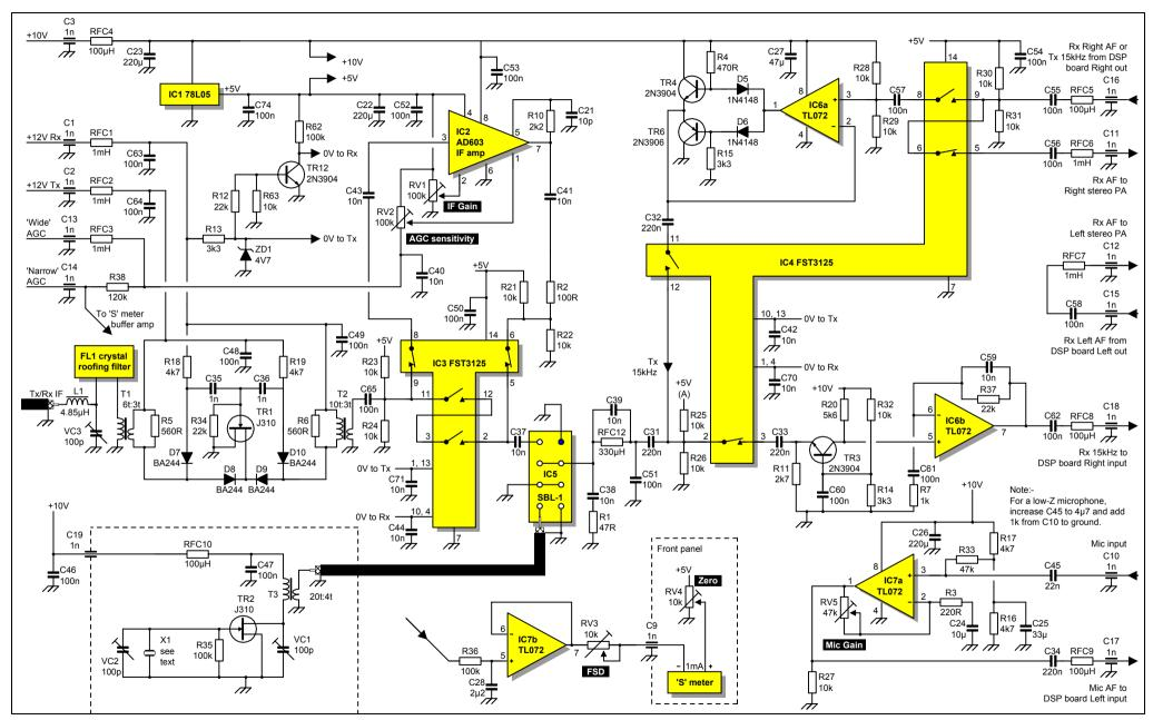
Fig 11: IF board circuit diagram. Takes an HF IF feed from a typical bi-directional mixer and post-mix amp and translates it to/from 15kHz. This board mounts back-to-back with the DSP board. All components are mounted on the track side except for the crystal filter FL1 and the SBL-1. The roofing filter is your choice and X1 must correspond. The switches in the receive path are shown as closed for illustration purposes only.
