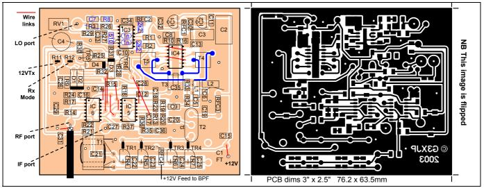
Fig 38: 'Magic Roundabout' component layout and PCB artwork. This board is designed to mate mechanically with the BPF assembly described next month. Components shown in blue are for the improved squarer. Track shown in blue may optionally be removed (see text) for the 2-transformer Hmode mixer.
