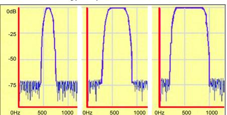
Fig 33: Plot of the Rx CW filters. This is the bank centred on 600Hz - and those on different centre frequencies are otherwise similar. Their widths are approximately 200Hz, 500Hz and 750Hz but this absolutely depends on where you measure them. This filter shape gives less ringing than a brick wall. Other filters in the receive path give a further theoretical 30dB of ultimate stop band.
