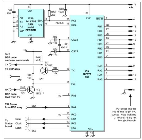
Fig 19: PicAdapter board circuit diagram. This board plugs into the 18-pin PIC socket on the original Pic 'N' Mix DDS board and upgrades the PIC to a more recent and versatile PIC, the 16F870.
