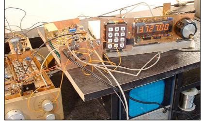
Early integration testing. Bottom left is my Third Method transceiver (borrowed front-
