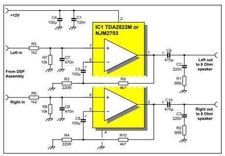
Fig 21: A suitable 1W + 1W stereo audio amplifier. Stereo balance and gain are controlled in DSP.
