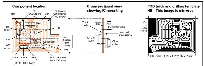
Fig 23: Double-sided PicAdapter board PCB. The cut-out is to give access to the existing programming socket. IC10 and IC9 should definitely be mounted in sockets. To achieve the clearance height required you may need to first fit an extra 18-pin socket into the existing Pic 'N' Mix socket - as a spacer. SIL plugs / sockets are used for the remaining leads - with the sockets soldered directly to the track.
