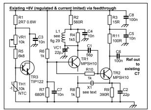
• Pic 'N' Mix now has Fig 27: Butler oscillator for either 5th or 7th overtone operation -
