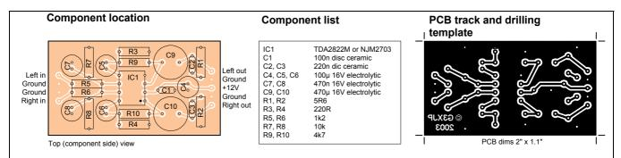
Fig 22: Double-sided stereo amplifier PCB. This is a 'conventional' board with components mounted on the top, the track underneath. The component side is completely unetched. No connectors are specified, but the relevant pads have a 0.1" pitch.
