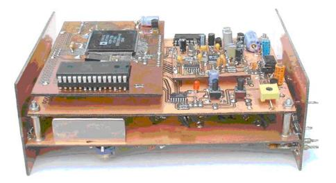
The DSP assembly. That is, the DSP mother board with CODEC and Processor daughters boards - mounted back-to-back with the IF board in its enclosure. The top, bottom and side screening panels are not fitted until after final test.
