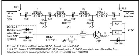
Fig 26: 26-40MHz injection filter to strip both unwanted high-order spurs and those at the IF from the DDS output - on the higher HF bands only. Not needed (ie switched out) on lower bands.
