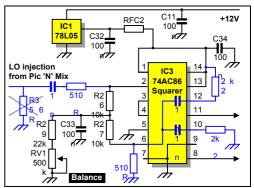
Fig 36: Modified squarer by I7SWX. The changes from fig 34 are shown in blue. Please note that neither the changed nor the incremental parts are included in the component list.
