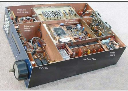
G3XJP's STAR built in a PCB enclosure - shown with all compartment cover-plates removed. The overall dimensions of the case are 310mm deep by 240mm wide by 85mm high. This generous size allows good *in situ* access to all the boards.
