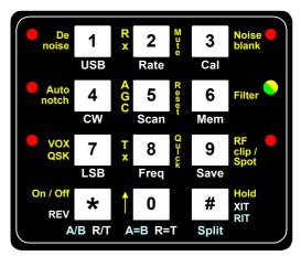
Fig 30: Keypad allocations and corresponding status LEDs. This is to scale and may be used as a keypad overlay. Note that this reflects recent developments.
