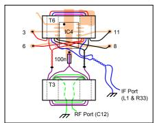
Fig 39: Details of T6 / T3 connections to each other and to IC4. This is not strictly to scale, but does show the correct relative positioning of the components. T6 and T3 will end up separated by about 6mm in practice. The T1 feedback turn is made from a length of miniature coax braid. Form the U-shaped primary turn - with plenty of excess lead length. Pierce and spread the braid to fill the tubular holes in the core - from both ends of the core. Make off the braid leads to the PCB track.
