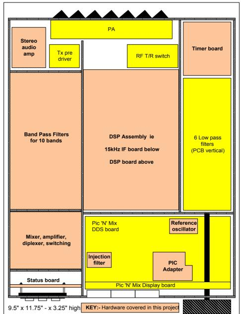
Fig 16: A possible transceiver enclosure illustrated at half scale. Mine is fabricated from 2mm doublesided fibreglass PCB stock. This gives excellent access from both sides.
