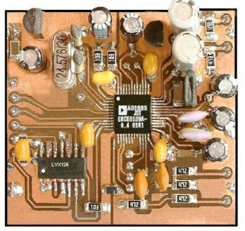
The completed CODEC board, illustrating the quality of PCB production available (0.2mm wide tracks at 0.5mm spacing) - using domestic kitchen resources. The CODEC chip is 7mm square.
