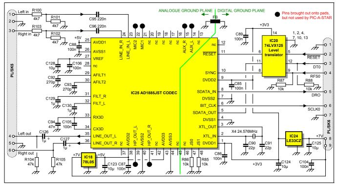
Fig 8: CODEC daughter board circuit diagram. Note that the ground plane is split between analogue and digital to minimise noise.
