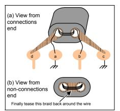
Fig 40: Transformer T1 detail. The pad designations correspond to those of fig 34.
