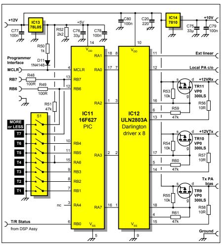
Fig 4: Timer board circuit diagram. This provides timed transitions between transmit and receive - in both directions. Sw1 allows you to set up the timing for your installation - and covers the range from slow relay-based RF T/R switching through to solid-state QSK.
