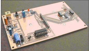
The DSP mother board, ready for daughter board fitting and test. Note IC8 and its associated components are located under the Processor daughter board. In fact, neither they nor IC22 need be fitted for standalone testing.
