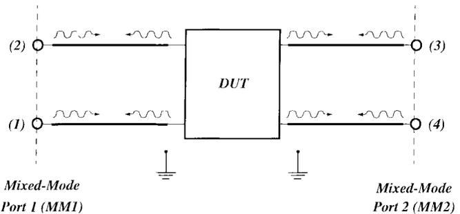
Fig. 1. Schematic of general two-port differential device.
