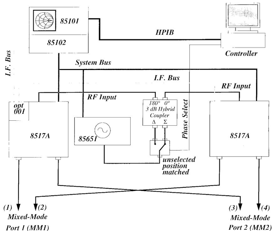
Fig. 2. Block diagram of PMVNA as implemented.
