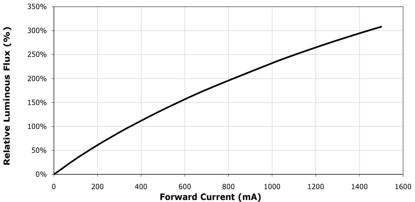
**RELATIVE RADIANT FLUX VS. CURRENT ( $T_j = 85\text{ }^\circ\text{C}$ ) - ROYAL BLUE**
