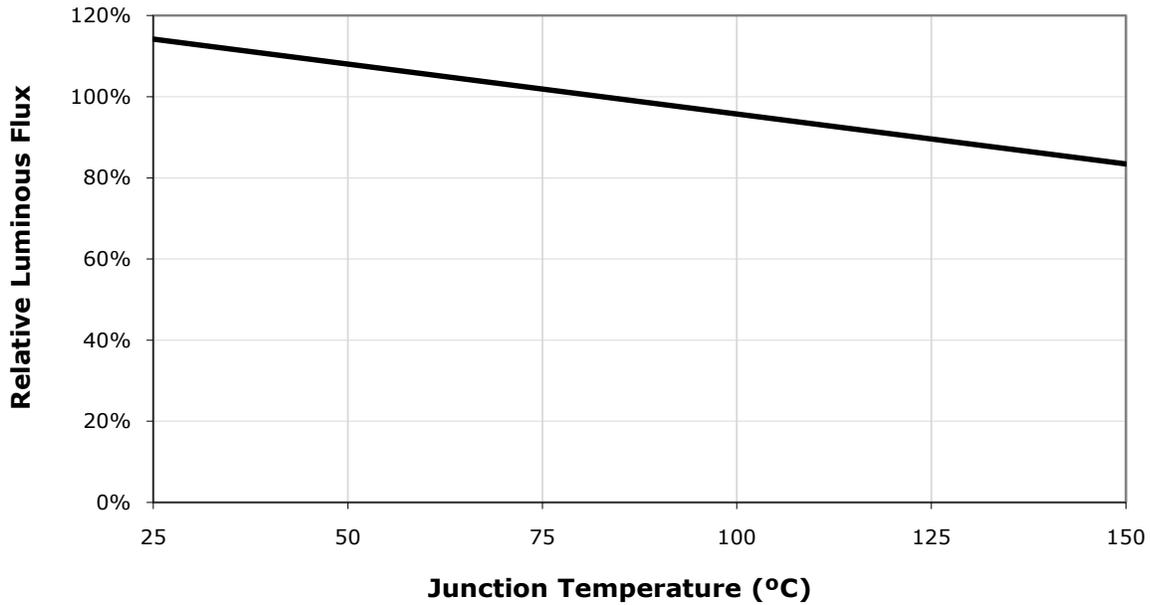
**RELATIVE RADIANT FLUX VS. JUNCTION TEMPERATURE ( $I_F = 350 \text{ mA}$ ) - ROYAL BLUE**
