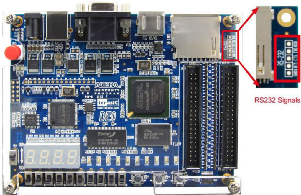
Figure 4-17 The placement of the RS232 signals
