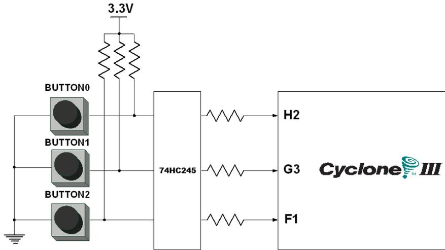
Figure 4-5. Connections between the pushbutton and Cyclone III FPGA
