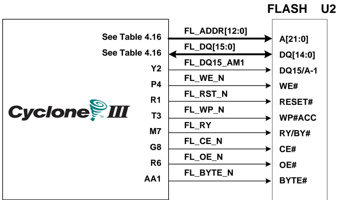
Figure 4-22 Connections between Flash and Cyclone III FPGA
