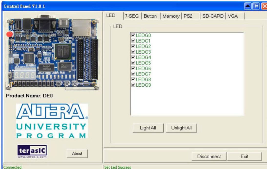
Figure 3-4. Controlling LEDs
