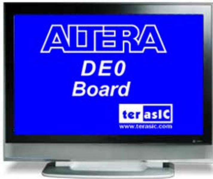
Figure 2-3 The default VGA output pattern.
