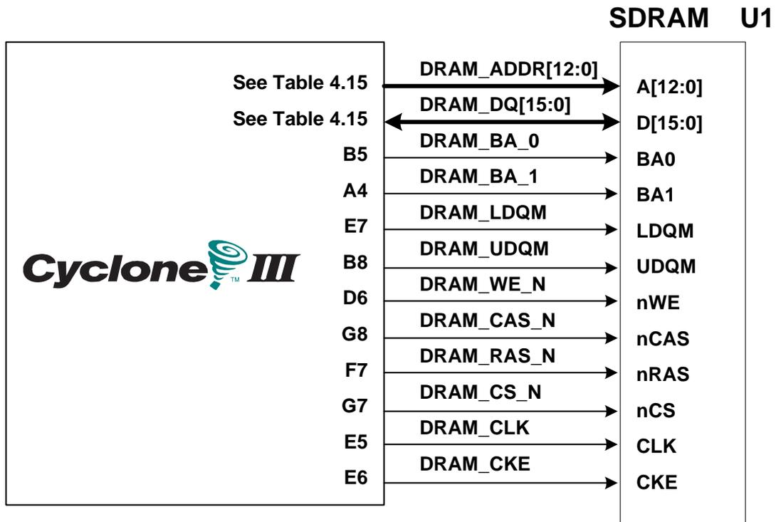
Figure 4-21 Connections between SDRAM and Cyclone III FPGA
