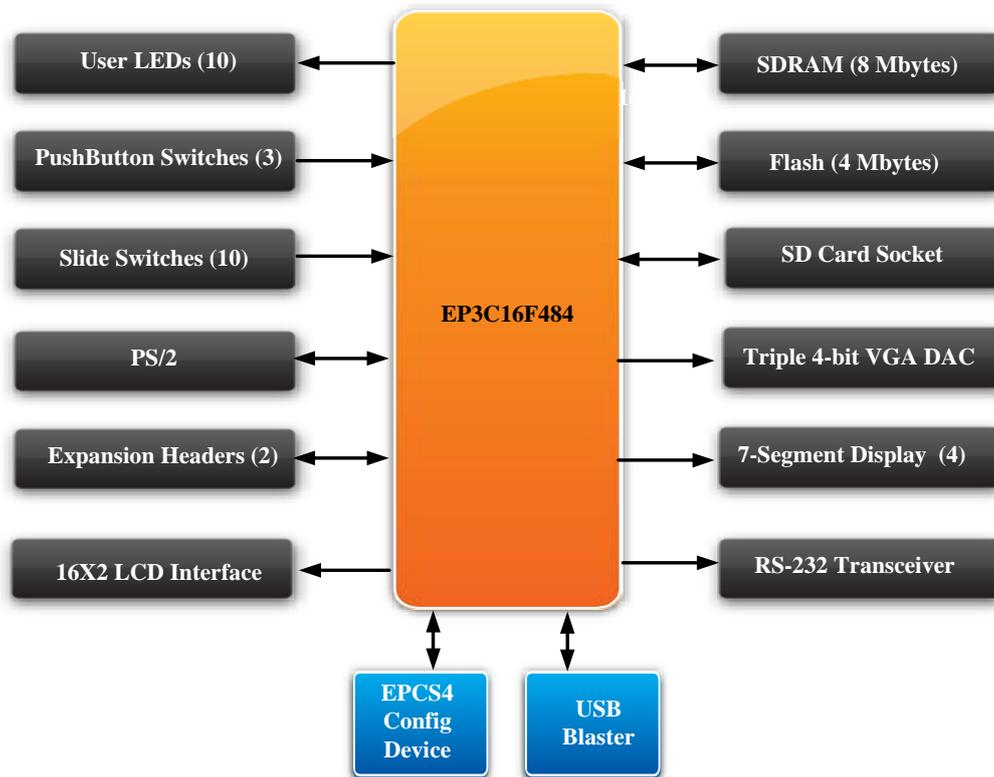
Figure 2-2 Block diagram of the DE0 board.
