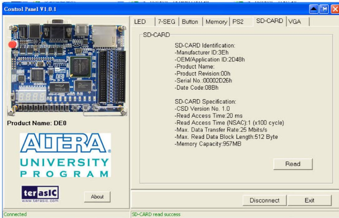
Figure 3-9. Reading the SD card Identification and Specification
