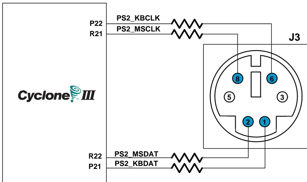
Figure 4-19 Connections between PS/2 and Cyclone III FPGA
