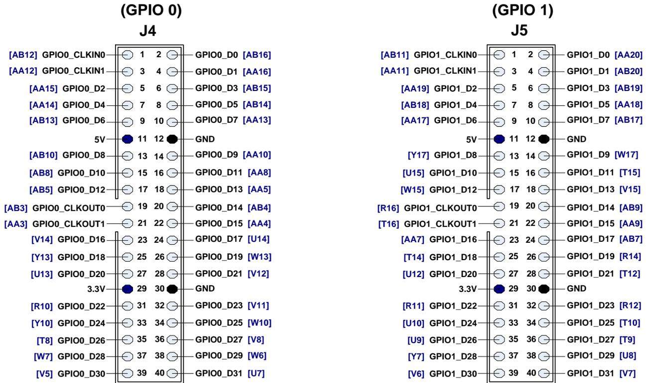
Figure 4-14 I/O distribution of the expansion headers
