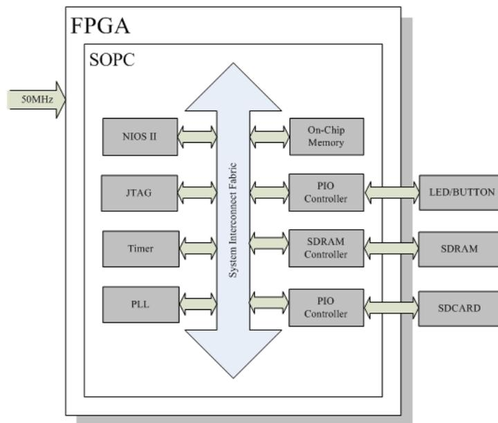
Figure 5-1 Block Diagram of the SD Card Demonstration
