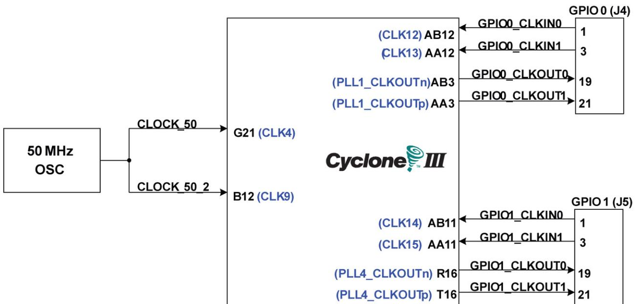
Figure 4-11 Block diagram of the clock distribution.
