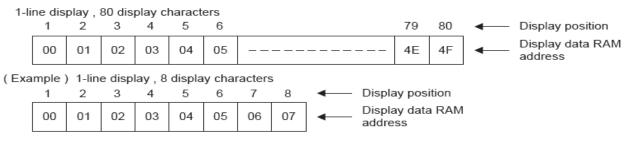
When the display shift operation is performed , the display data RAM's address moves as :
