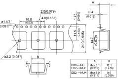
Relay orientation mark and tape carrying direction.
