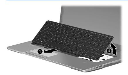
Rotate the keyboard until it rests on the palm rest (1), and then disconnect the keyboard cable by lifting the keyboard connector latch (2), and then disconnecting the keyboard cable from the system board (3).
