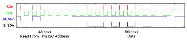
**Example 2:** This example shows how to read two bytes from the HMC6352 (slave). The slave continues to hold the SDA line low after the acknowledge bit because the first bit of the data bytes is zero.
