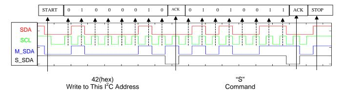
I<sup>2</sup>C bus control can be implemented with either hardware logic or in software. Typical hardware designs will release the SDA and SCL lines as appropriate to allow the slave device to manipulate these lines. In a software implementation, care must be taken to perform these tasks in code.
