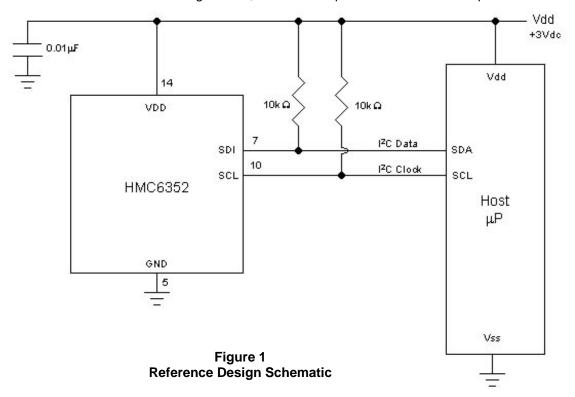
The  $0.01\mu F$  supply decoupling capacitor in this reference can be omitted if another supply filter capacitor is already included in the overall circuit design. If the supply traces extend beyond a couple inches to the HMC6352, it is advisable to add a local supply decoupling capacitor near the HMC6352 to retain optimum circuit stability.
