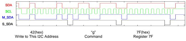
**Example 4:** This example shows how to write to a RAM register in the HMC6352 by sending the "G" command, the register address 7F(hex), and the data byte 55(hex) to the HMC6352 slave.
