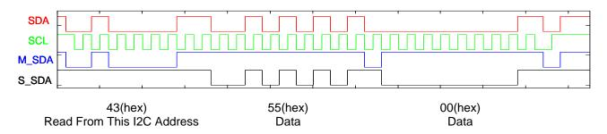
**Example 3:** This example shows how to command HMC6352 to read a RAM register by sending the "g" command and the register address 7F(hex). Note that this example does not show the process of reading the answer. See example 1 for reading a byte.
