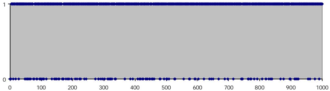
Fig 7: Loss of IEEE802.15.4 frames with a high activity IEEE802.11 DSSS overlapping channel: The x-axis shows the number of the frame; a "0" on the y-axis indicates a successful transmission, a "1" stands for a frame loss
