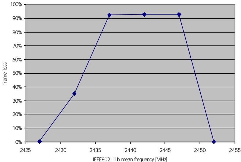
Fig 9: Loss of IEEE802.15.4 frames with a high activity IEEE802.11 DSSS; varying 802.11 channel, 802.15.4 channel kept constant at 2440 MHz
