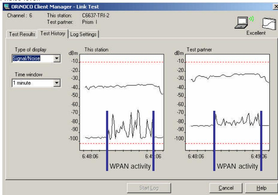
Fig 11: Increased noise level of IEEE802.11 in times of IEEE802.15.4 activity. This station is the Notebook with the Orinoco WLAN card very near to the IEEE802.15.4 (< 10 cm), the test partner is the router in a distance of approx. 50 cm. The upper curve shows the signal level, the lower curve the noise level.
