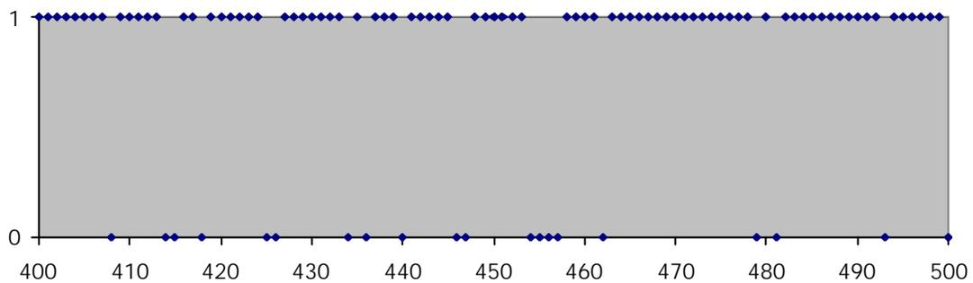
Fig 8: Loss of IEEE802.15.4 frames with a high activity IEEE802.11 DSSS overlapping channel: Extract from fig. 7
