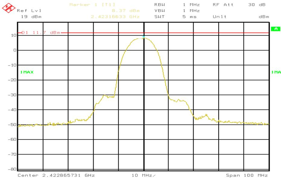
Fig 6: Frequency behaviour of a IEEE802.11 DSSS-transmission (courtesy of Tenovis)
