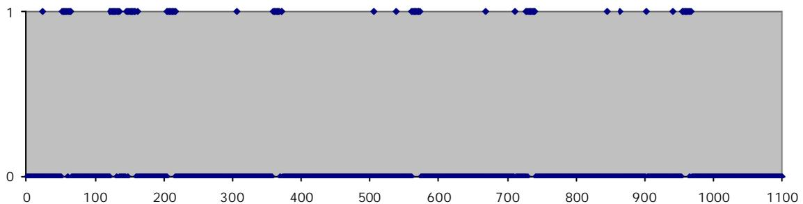
Fig 16: Loss of IEEE802.15.4 frames with Bluetooth interference
