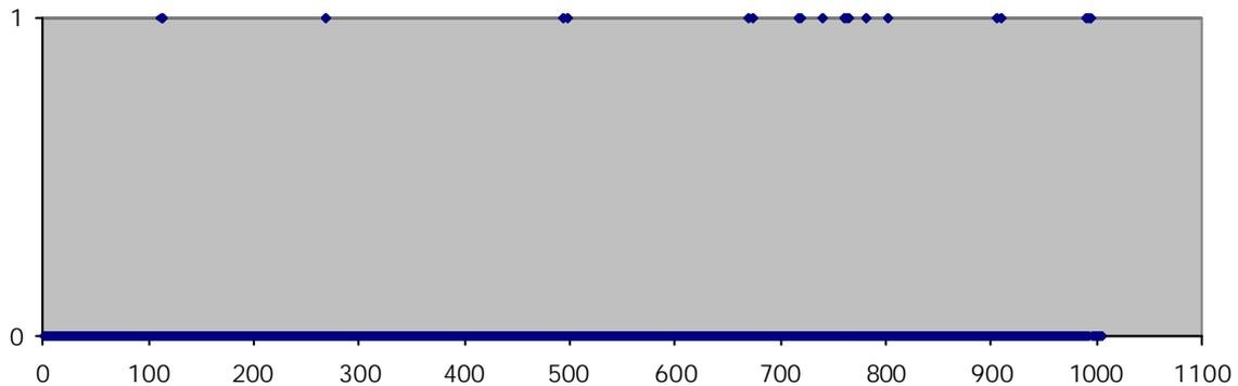
Fig 18: Loss of IEEE802.15.4 frames when used on top of a microwave oven
