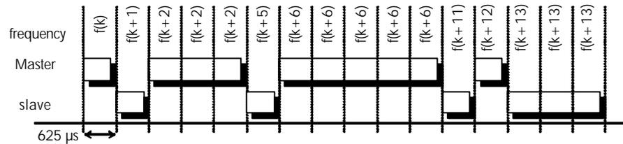
Fig 15: Frequency Hopping of Bluetooth systems
