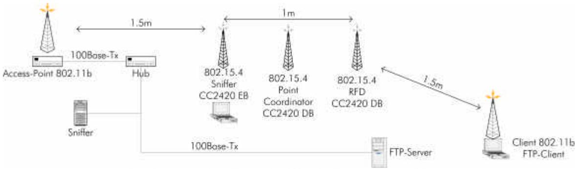
Fig 5: Environment for IEEE802.11b DSSS and IEEE802.15.4 compaibility tests
