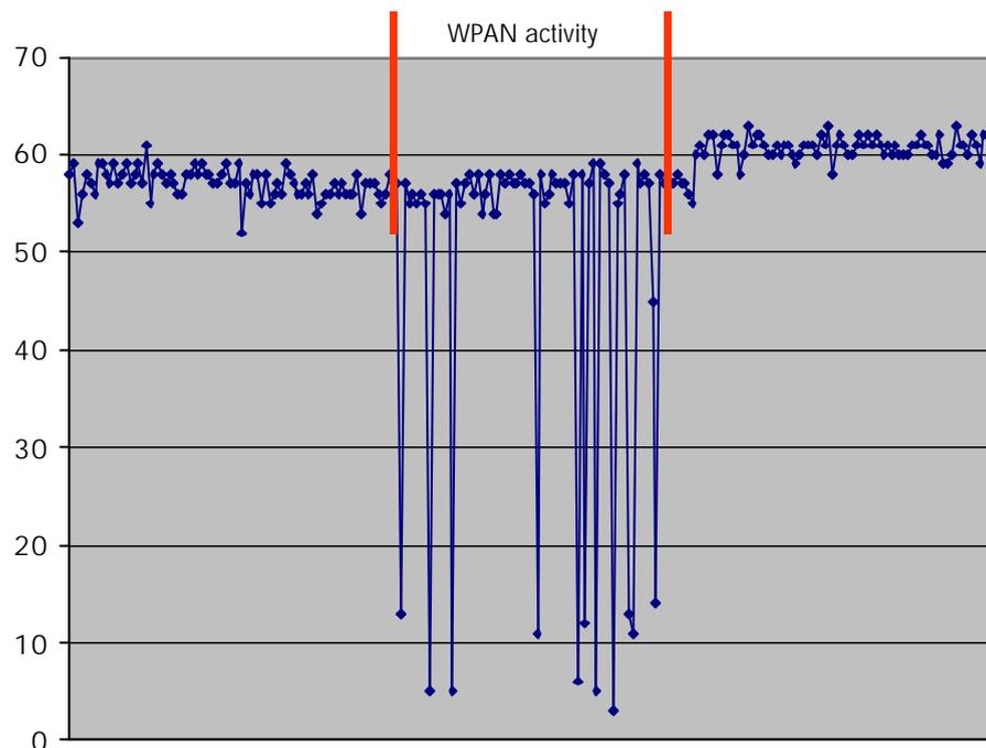
Fig 12: Reduced signal to noise ratio of IEEE802.11 in times of IEEE802.15.4 activity.
