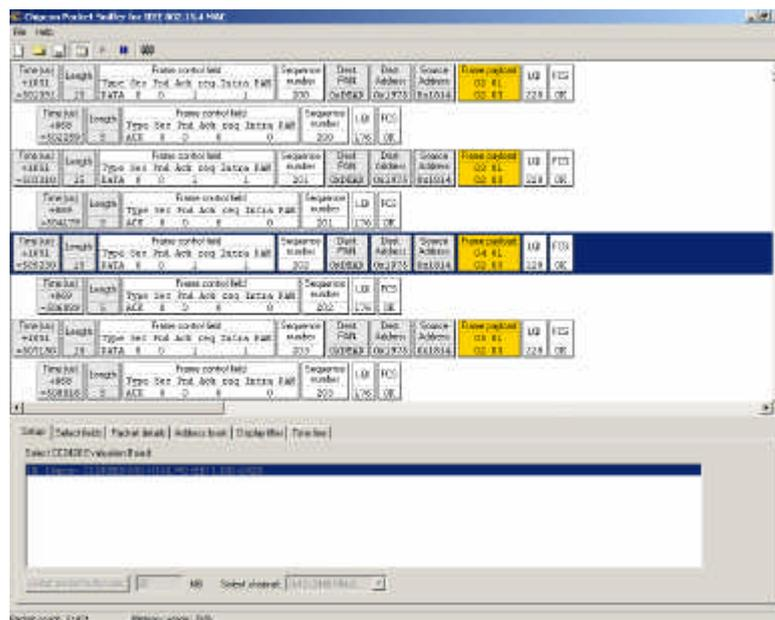
Fig 2: Timing behaviour of IEEE802.15.4 at maximum load
