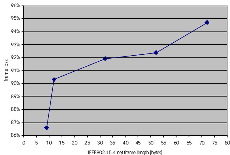
Fig 10: Loss of IEEE802.15.4 frames with a high activity IEEE802.11 DSSS; varying the IEEE802.15.4 frame length; the 802.11 channel is kept constant at 2437 MHz, the IEEE802.15.4 channel is at 2440 MHz
