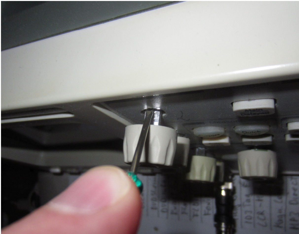
Fig 3: Lever off the knob
