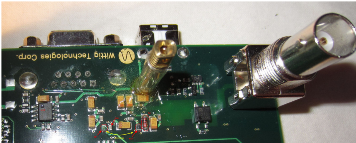
Fig 10: Mainboard front side and external trigger BNC connector
