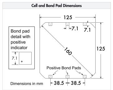
Bond pad area dimensions are 7.1mm x 7.1mm Positive pole bond pad side has "+" indicator on leftmost and rightmost bond pads.
