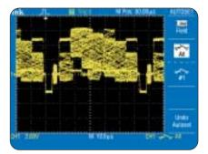
Pulse-width and field- and line-selectable video triggers make the oscilloscope ideal for a wide range of applications.
