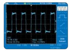
Automatically detects sine waves, square waves and video signals, with readouts of relevant measurements and additional user-selectable views of the signal.
