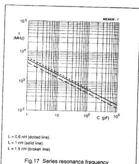
Fig.17 Series resonance frequency as a function of capacitance.
