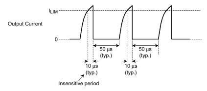
The set limit is 5 A (typ.) as a design target value. The distributions shown below exist because of the variations in thermal characteristics of different ICs. These distributions should be fully considered in the motor torque design.
