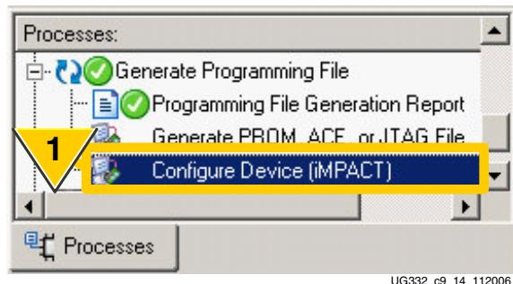
*Figure 9-7: Double-click Configure Device (iMPACT)*
