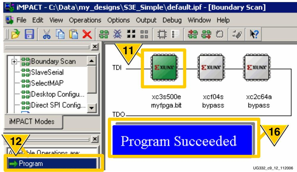
Figure 9-14: Double-Click Program to Configure FPGA via JTAG
