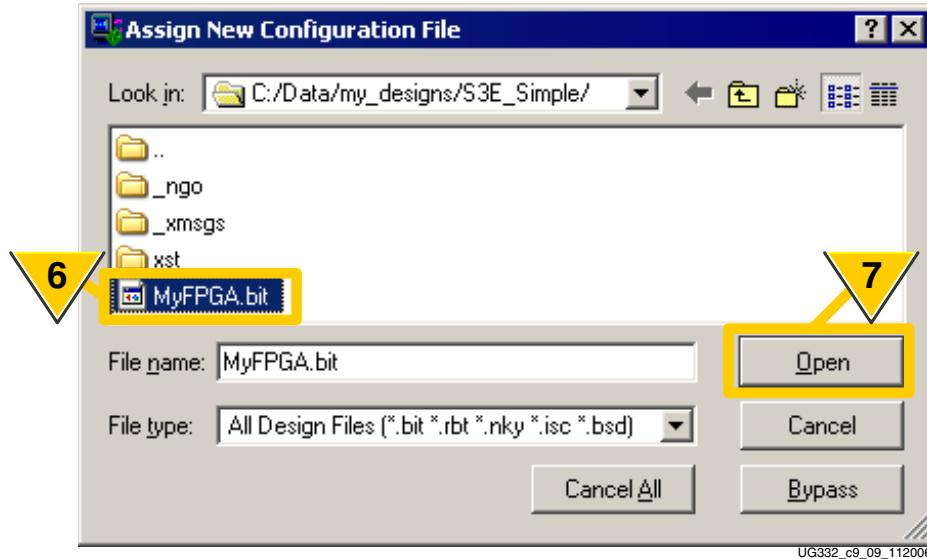
Figure 9-10: iMPACT Prompts for FPGA Bitstream
