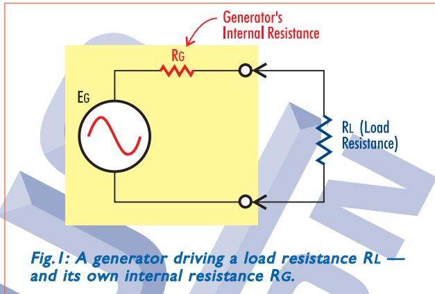
**Fig.1:** A generator driving a load resistance  $R_L$  — and its own internal resistance  $R_G$ .
