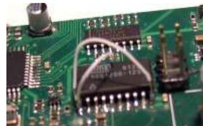
Figure 3 - Connecting all the reset pins to GND
