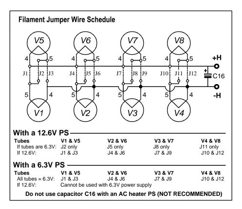
Since one triode stands atop another, the heater-to-cathode voltage experienced differs between triodes. The safest path is to reference the heater power supply to a voltage equal to one fourth the B+ voltage; for example, 75V, when using a 300V power supply. The <sup>1</sup>/<sub>4</sub> B+ voltage ensures that both top and bottom triodes see the same magnitude of heater-to-cathode voltage. The easiest way to set this voltage relationship up is the following circuit:
