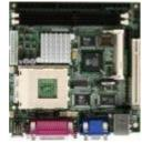
positioned" mini-ITX SBC (single-board computer) that can be used to create a media server. The EMB-820T is based on AMD's Athlon-family embedded processors, and features TV output and 5:1 surround sound, ...
