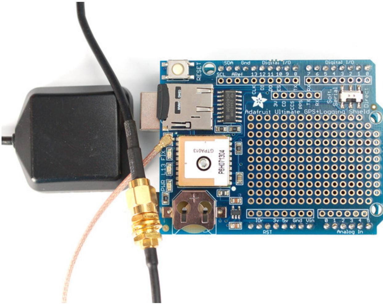
Active antennas draw current, so they do provide more gain but at a power cost. Check the antenna datasheet for exactly how much current they draw - it's usually around 10-20mA. (<http://adafru.it/960>)
