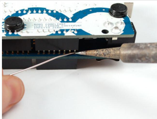
Turn the Arduino upside down so its resting on the long parts of the stacky headers and solder them from below.
