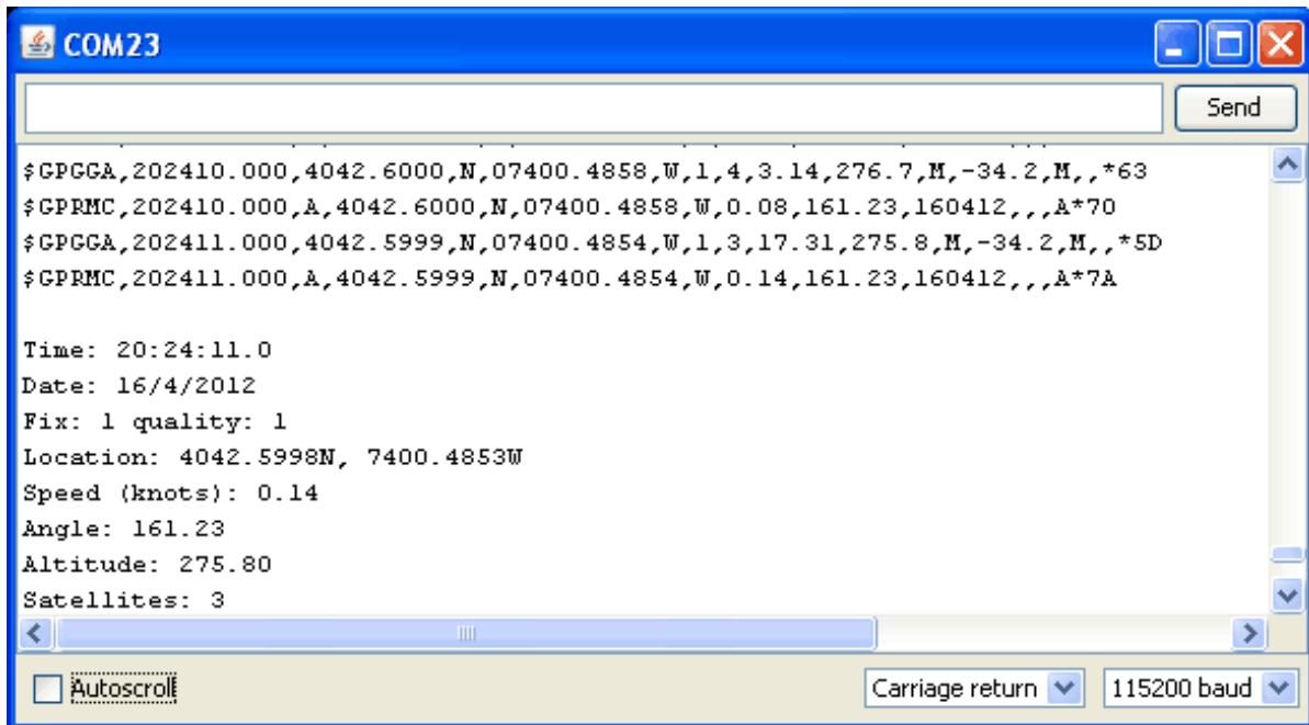
In this sketch, we can either use interrupts and call **GPS.read()** within a once-a-millisecond timer (this is the same timer that runs the **millis()** command) or we check **GPS.read()** in the main loop constantly. Then in the main loop we can ask if a new chunk of data has been received by calling **GPS.newNMEAReceived()**, if this returns **true** then we can ask the library to parse that data with **GPS.parse(GPS.lastNMEA())**.
