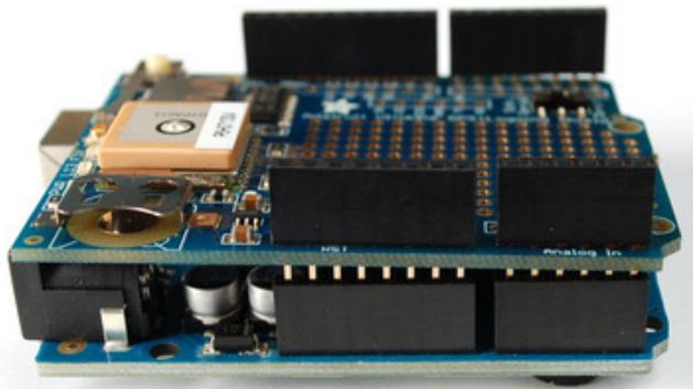
Fit the long pins through the pads until they slot into the Arduino. Depending on which version/type of Arduino you may need to use 2 x 8pin and 2 x 6pin *or* 1 x 10pin, 2 x 8pin and 1 x 6pin.
