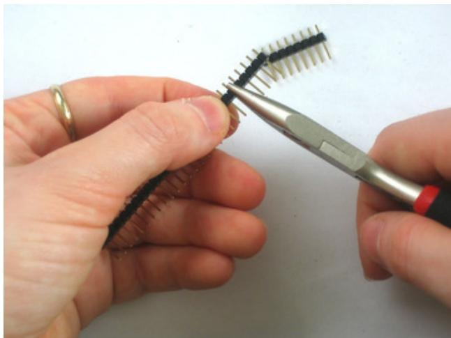
If you want to go with male headers, break off the 36-pin long stick into either 2 x 8pin and 2 x 6pin or 1 x 10pin, 2 x 8pin and 1 x 6pin (depending on how many headers your Arduino has and which version it is)
