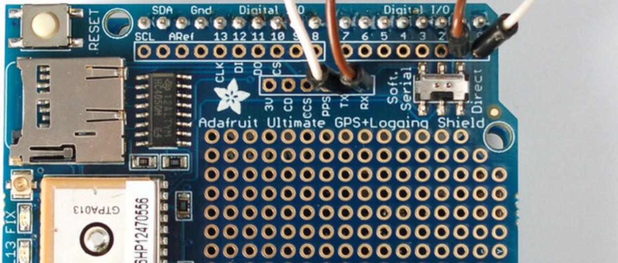
Finally upload the **Adafruit\_GPS->leo\_echo** sketch to the Leonardo, this will shuffle data from the GPS to the USB port
