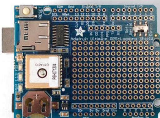
If you want to go with stacking headers, place the the shield PCB on top of the Arduino
