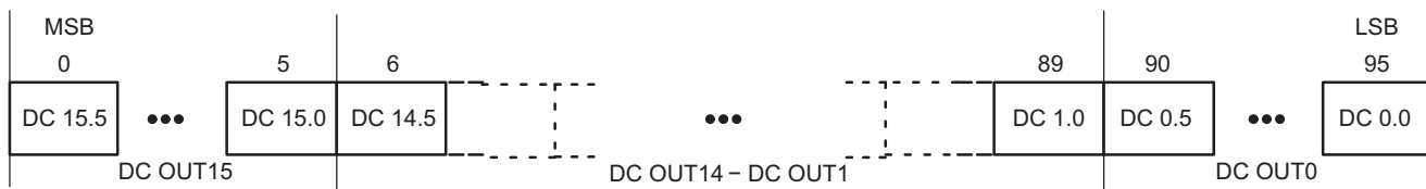
Figure 15. Dot Correction Data Packet Format
