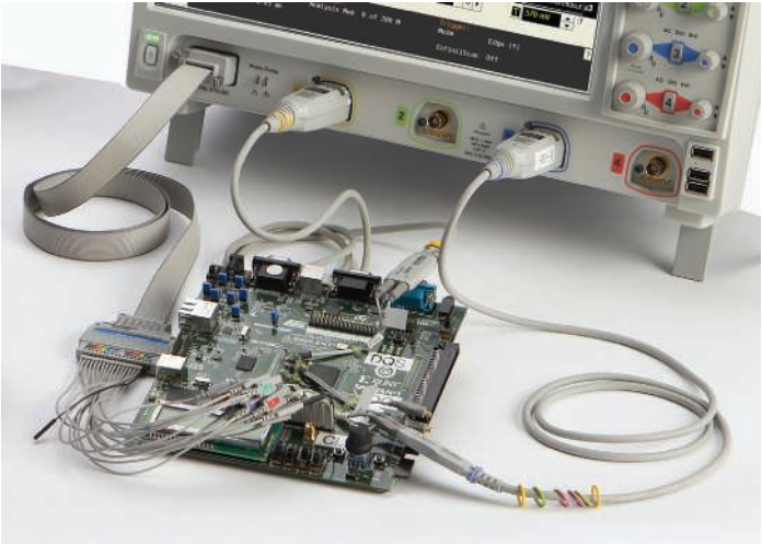
Designing with Xilinx FPGAs? Use the FPGA dynamic probe for rapid internal FPGA measurements. Using I 2 C, SPI, RS-232, or low- or full-speed USB? Use the digital channels to acquire and decode these buses, preserving analog channels for other time-correlated measurements.
