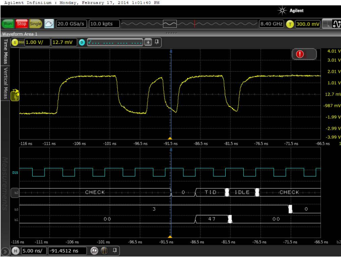
Use the timing channels to evaluate control signal relationships and data buses up to 16 bits wide. Use symbols to more quickly interpret waveforms.
