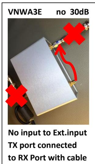
**Test of the internal TCXO with nothing connected to the Ext. input. A cable connected between RX or TX port and in the Frequency meter panel Source selected to S21**
