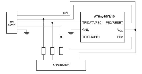
Refer to the corresponding device datasheet for more details on the TPI protocol.
