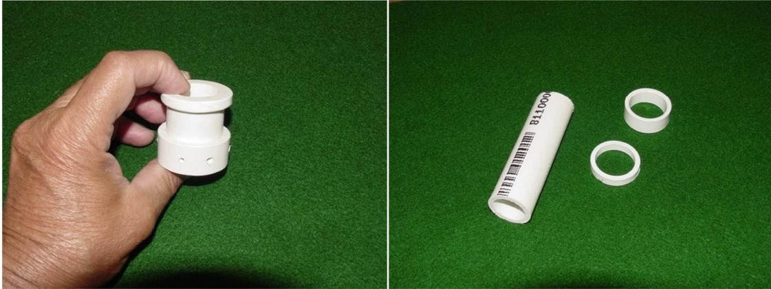
The coil body is 1" id and 1.75" in overall length. It is made of PVC plumbing fittings, cut to fit. Note: Use any 1" pvc fitting, like a coupler for the rings. Use the thinner wall pvc pipe, 200 psi, and not the thicker pipe, for the body.
