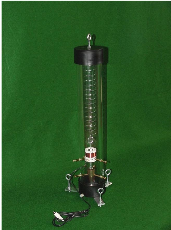
The original Slinky vertical seismometer was encased in 3" ABS plumbing pipe.
