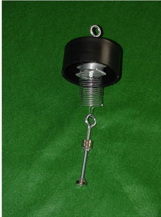
The spring is suspended from a ¼" 20 x 4" eyebolt, nuts, and the 3" ABS cap.
