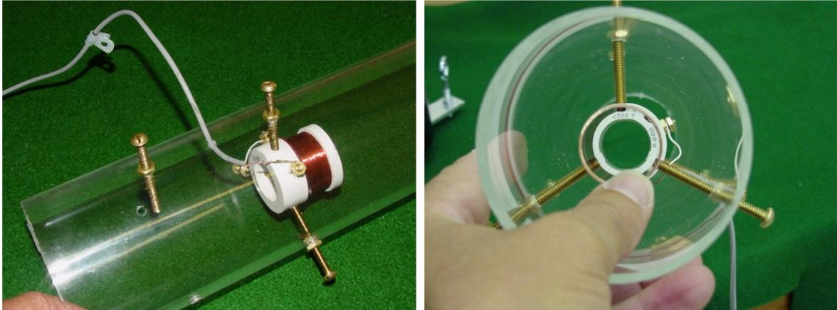
Drill a hole for the cable, to fit the cable diameter.
