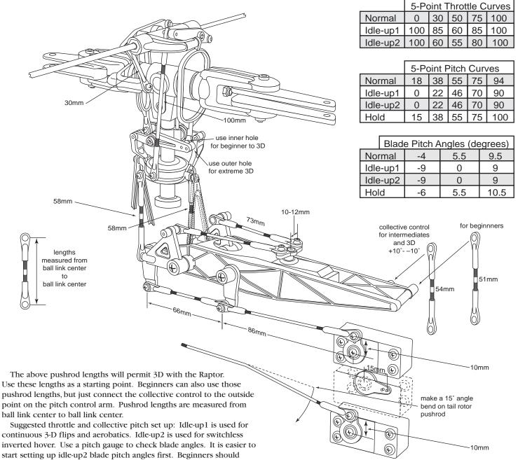
inverted hover. Use a pitch gauge to check blade angles. It is easier to start setting up idle-up2 blade pitch angles first. Beginners should inhibit idle-up1, idle-up2 and throttle hold. Beginners should only use the Normal mode values. The model should hover at around 1550 rpm in Normal mode, and flies at 1800 in idle-up1. Rotorspeed can be checked using TTR2000 MTF-301 helicopter tachometer.
