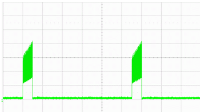
Blockierstrom @ 24 V ( I = 200 \text{ mA/div} ; t = 1 \text{ s/div} )
