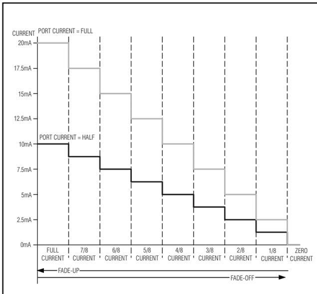
Figure 6. Output Fade DAC (Global Current = 0x07)
