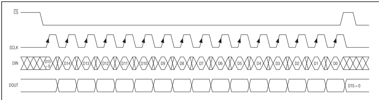
Figure 11. 16-Bit Write Transmission to the MAX6966/MAX6967
