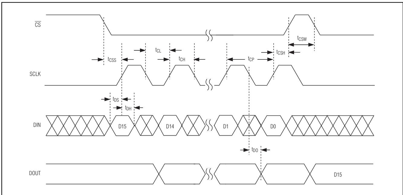
Figure 10. Timing Diagram
