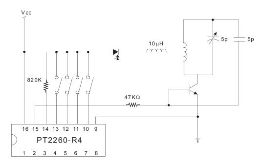
UHF Band 4-Data Transmitter Circuit is recommended.
