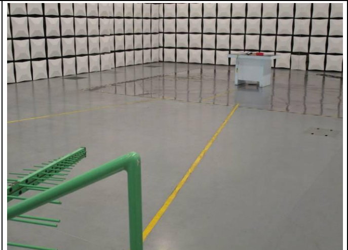
Figure 4: Measurement radiated emission at SC-620
