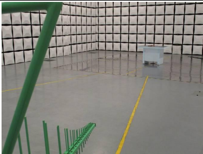
Figure 3: Measurement radiated emission at Q6 plus
