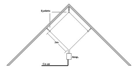
three eyelets in the rafters to give an approximate diamond shape. Since my house is facing due N/S, the eyelets were placed that the direction of the loop is pointing NE/SW.
